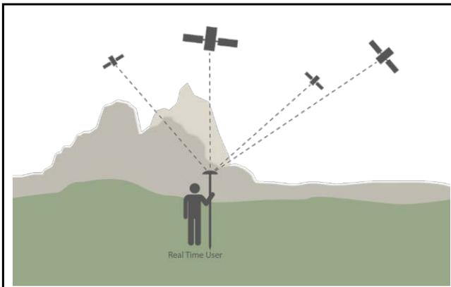
Real-time GPS: The receiver directly calculates its position based on the received satellite signals (illustration source : [swisstopo](http://swisstopo))
