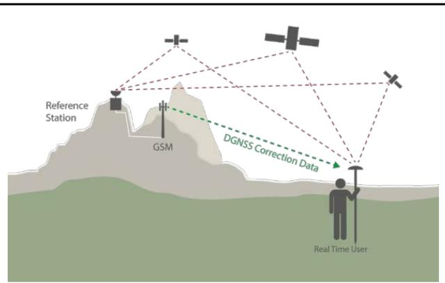
Real-time differential GPS: A reference station, whose position is known, calculates its position on the basis of received satellite signals. From these two positions, one known and the other calculated, it is possible to calculate a position and/or correct locational errors (illustration source : [swisstopo](http://swisstopo))
